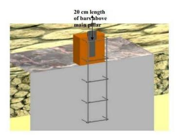
$\label{eq:action} A'Survey Reference Mark' made of Gun Metal/brass as shown in the figure will be embedded at the centre of pillar, flushed with the top surface of the pillar.$
